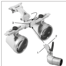
Fig. 6 Fitting the headband rheostat
